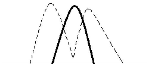
Fig. 3. Histogram of gray levels of true boundary (solid curve) and histogram of “double responding” edge points (two dashed curves) of each object in 2D image.
