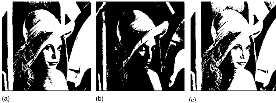
Fig. 11. Binary images of the girl: (a) Otsu method ( t = 101 ); (b) Kapur, Sahoo and Wong method ( t = 139 ); (c) our method ( t = 90 ).
